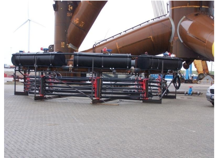
....and the upper tube system including uplift bodies, which couldn't be put into use, designed by Hydrotechnik Lübeck and MENCK
